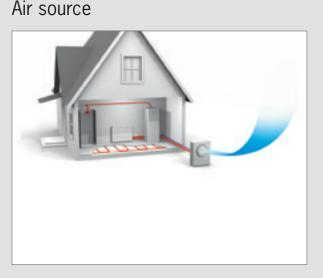
With an air source heat pump there is no need to dig or drill. Instead the energy is sourced straight from the surrounding air.
