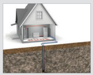
The vertical ground loop collects solar energy stored in the bedrock. A hole is drilled into the bedrock and a pipe is installed to a depth of between 100 and 200 metres. The exact depth depends on the house, size of heat pump and surrounding conditions.
