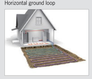
The horizontal ground loop collects solar energy stored in the ground, near the surface. If the bedrock is too deep down, or if you don't want to drill for other reasons, this is a good option.
